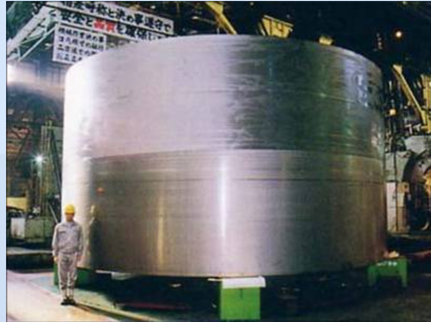
Forging for reactor pressure vessel: 24' diameter x 13' high: 127 Tons
